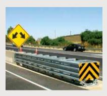
The Smart Cushion® crash attenuator is a revolutionary, speed-dependent product that varies stopping resistance during an impact. The Smart Cushion® crash attenuator allows lighter and slower-moving vehicles to have longer ridedown distances and lower ridedown g-forces.
